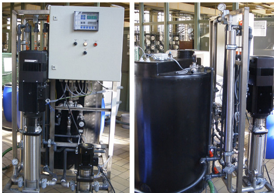
Fig. 2. Membrane filtration equipment (frontal and lateral views).
